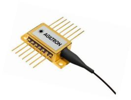
The 980nm series laser diodes are fabricated in a hermetically sealed 14-pin butterfly package. The laser diodes contain a monitor photodiode, thermoelectric cooler (TEC), and a thermistor to secure high-quality laser performance. Our laser products are Telcordia GR-468 qualified and in compliance with RoHS Directives.
